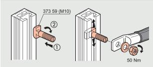
The lugs or flexible bars connect directly with no need to add washers or spacers
