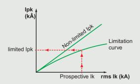
The table below gives the limited peak value (Ipk) directly for the maximum prospective short-circuit value equal to the breaking capacity (Icu) of the device
