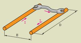
D: length of the conductor (distance between supports in the case of bars)
