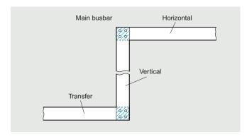
For branch busbars, the contact area can be smaller, complying with the condition  $Sc > 5 \times Sb$ . For equipment connection plates, contact must be
