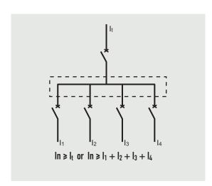
In practice, it is possible to select one or more distribution blocks with a lower nominal current if the downstream circuits are not on-load simultaneously (bulking factor) or are not 100% on-load (diversity coefficient) (see Book 2). 160 A 125 A 125 A  $|_1 + |_2 + |_3 + |_4 = |_4$
