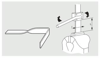
^ Creating a twist. The length L of the twist is at least twice the width I of the bar
