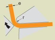
Bending on bending machine: r = 1 to 2e
