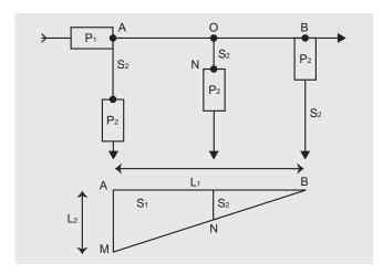
$\mathsf{S}_1$  corresponds to the cross-section of the main conductor and  $\mathsf{S}_2$  to the cross-section of the branch conductor.
