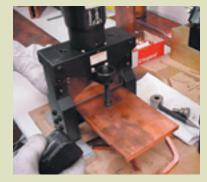
Bending a 10 mm thick copper bar on a portable hydraulic tool
