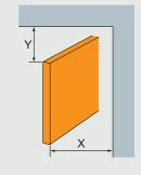
Induction is higher facing the flat surface of bars (distance X).
