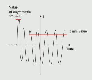
The relationship between the peak value and the rms value of the prospective short-circuit current is defined by the coefficient of asymmetry n:
