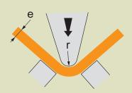
Bending on V-block:  $r \min = e$
