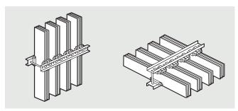
^ Bars mounted edgewise in vertical or horizontal busbars: supports in horizontal position
