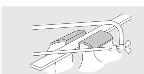
^ Sawing (8D medium tooth) in a clamping vice
