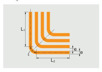
The bars are separated by their thickness "e". The total centre line length before bending is the sum of the straight parts (L1 + L2) that are not subject to any distortion and the length  $\ell$  of the curved elements on the neutral line (in theory at the centre of the thickness of the metal).
