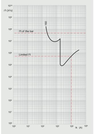
Example: using a 12 x 4 mm rigid flat bar for 160 A permissible  $I^2$ t of the bar: 4.7 x  $10^7$   $A^2$ s Prospective rms Ik: 10 kA ( $10^4$  A)
