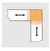
sanding (240/400 grain) can be carried out, complying with the direction of sanding so that the "scratches" on bars that are in contact are perpendicular.
